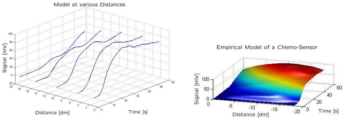
Figure 10: Empirical Model of a Chemical Sensor
