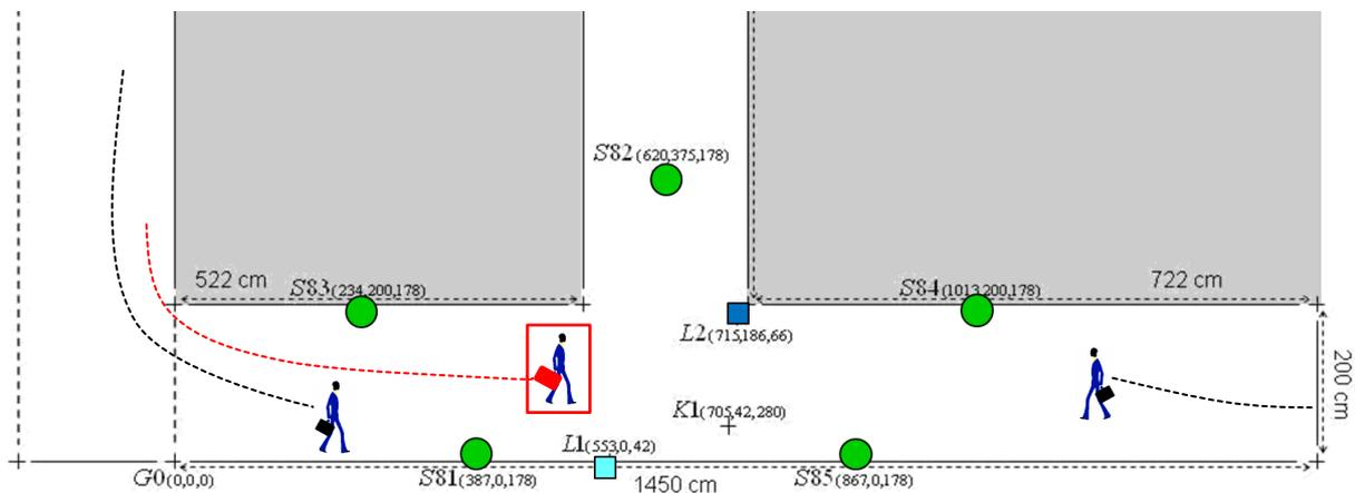
Figure 3: Experimental Corridor with five Chemical Sensors
